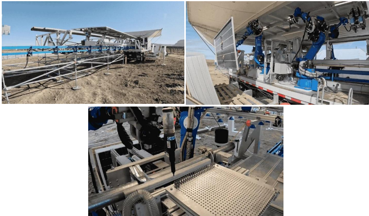
Figure 11: Solar Installation Robot from Charge Robotics (Charge Robotics)
